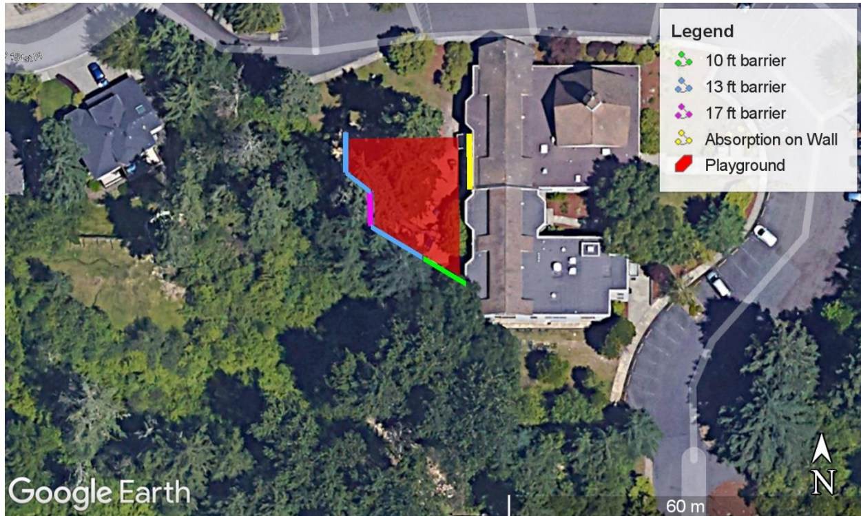
Figure 6. Minimum noise barrier heights
